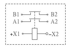
Note: A1, A2 are load terminals, +X1 (red wire), -X2 (black wire) are coil leads, B1 (white wire) is auxiliary contact, and the load terminal has no polarity (or polarized products have polarity), Coil has polarity, auxiliary contact has no polarity.
